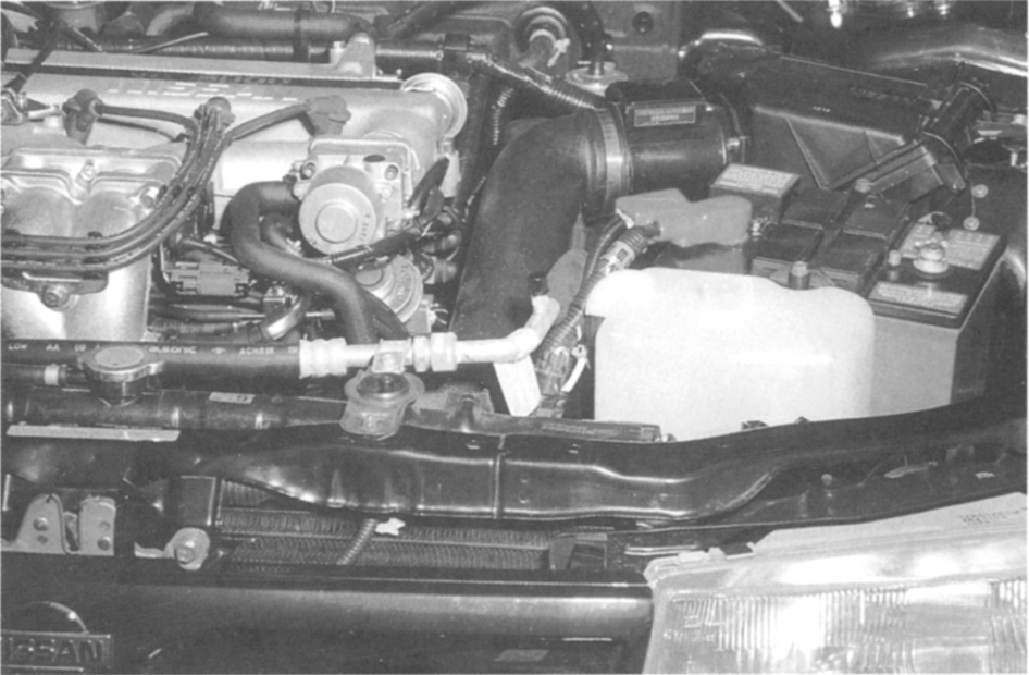
Fig. 16. The Powerbeat battery looks like a conventional battery; it is designed to be a 'drop-in' replacement for existing batteries. This is possible with modern vehicles that divide the starter motor cable from the auxiliary power harness at the battery's terminals.
